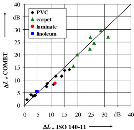
**Figure 9:** Deviation of  $\Delta L_w$  [dB], timber: COMET vs. ISO procedure
